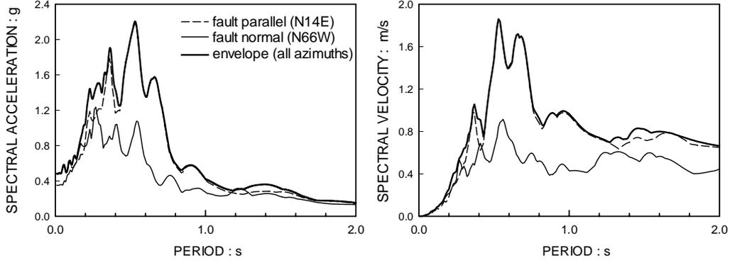
**Figure 3. Response spectra of Hospital motion at different orientations;  $\zeta = 5\%$**
