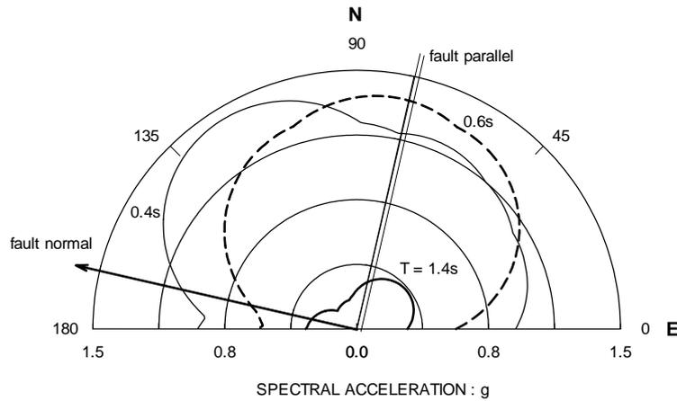
**Figure 4. Polar representation of spectral accelerations for Hospital motion at different periods;  $\zeta = 5\%$**
