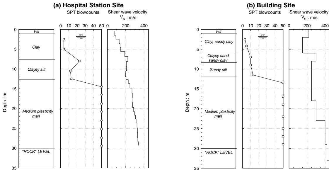
Figure 8. Soil profile and properties at Lefkada Hospital station (a) and building site (b).
