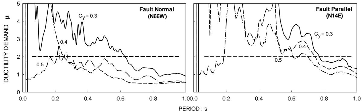
**Figure 5. Ductility spectra of Lefkada Hospital motion at orientations normal and parallel to fault.**
